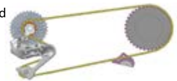
Simulation model of the bicycle drivetrain
