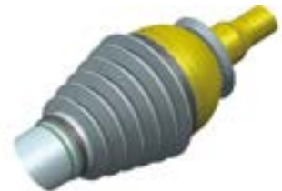
Rigid model of the boot on the CV half-shaft
