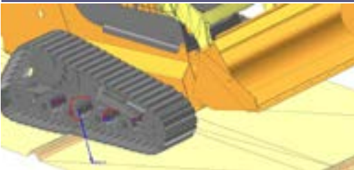
Force/Torque applied to rollers and idlers are displayed.
