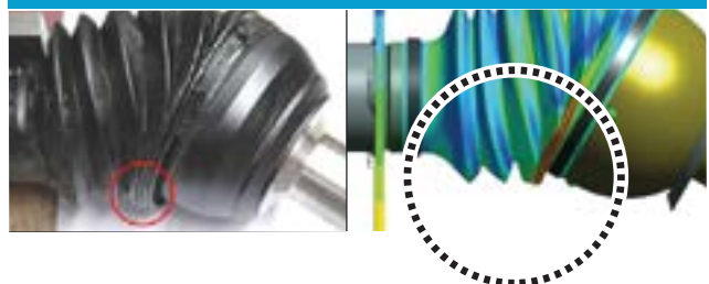
RecurDyn correctly predicted the number of collapsed folds
