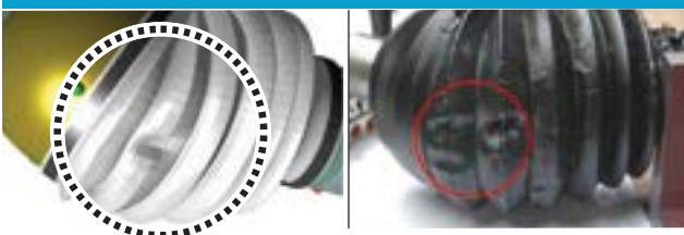
RecurDyn correctly validated the formation of dimples
