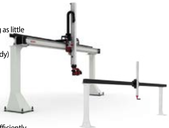
Digital twin model of the linear handling axes
