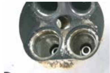
The carbon deposits around the engine inlet ports
